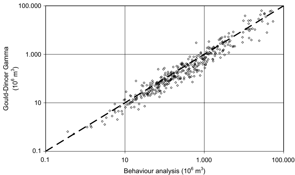
Fig. 4. Comparison of Gould–Dincer Gamma reservoir estimates with Behaviour estimates for \alpha = 0.75 and 95% reliability. The analysis was restricted to 0.4 < m < 1.0 , n_{crit} > 1 year and annual coefficient of skewness of streamflow < 4.0 . The 1:1 line is dashed.
